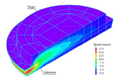
Figure 2. Flow field between the target and the substrate (CFD model)
