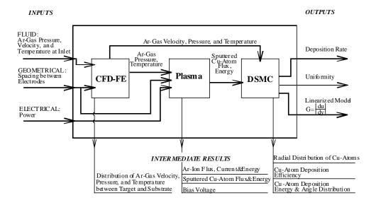
Figure 6. Virtual integrated prototype for GMR
