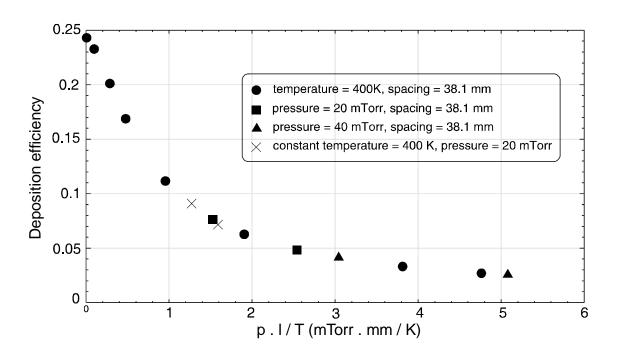
Figure 5. Deposition efficiency calculated from DSMC transport model
