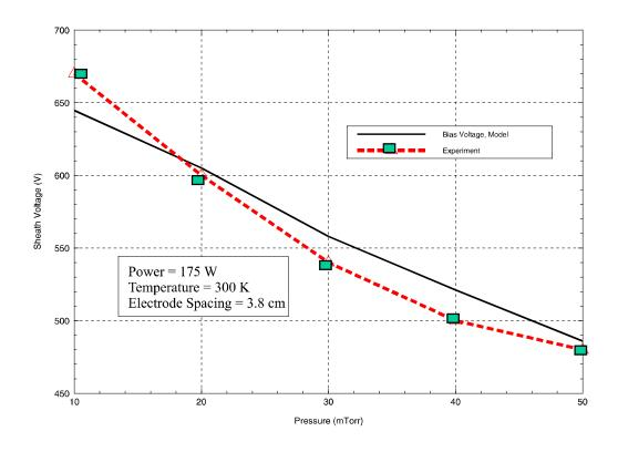
Figure 3. Experimental validation of the plasma model
