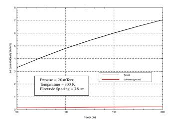
Figure 4. Effect of power on the ion current density (Plasma model)
