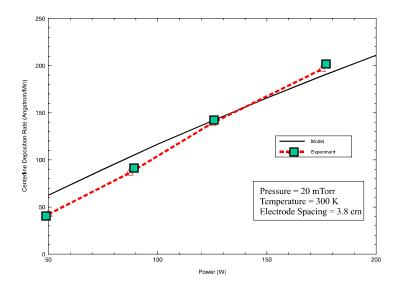
Figure 7. Experimental validation for deposition rate vs. power (Integrated model)
