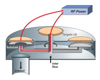
Figure 1. Schematic depiction of the GMR chamber used by NVE (PE2400 Sputtering System)
