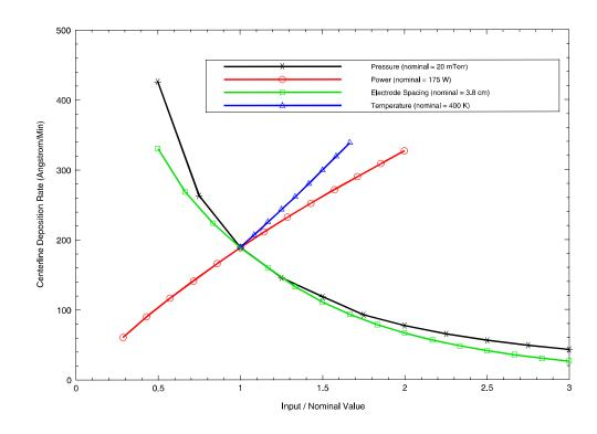
Figure 8. Sensitivity of deposition rate to the input process variables (Integrated model)
